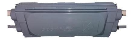
The TBE-I2 Façade Tapping Box is used to distribute the fibres from an in-line Retractanet/Verticasa cable into drop cables or tubes, for routing to a customer premise. It is sealed to IP55, enabling it to be mounted in the façade/aerial environment. It has the capacity to accommodate an in-line cable of up to 13 mm in diameter. The closure also provides the facility to accommodate two fusion splices. The closure is re-enterable and can be supplied in grey.
