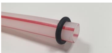
Figure 9: duct gasket insertion.
