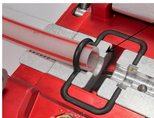
Figure 10: minitube proper insertion.
