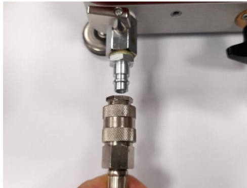
Figure 15: connecting the air hose to the compressed air connector
