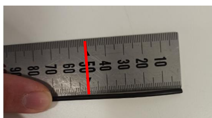
Figure 35: cutting the linear gasket.
