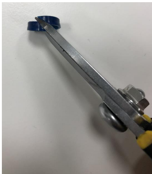
Figure 22: cut gaskets diagonally.
