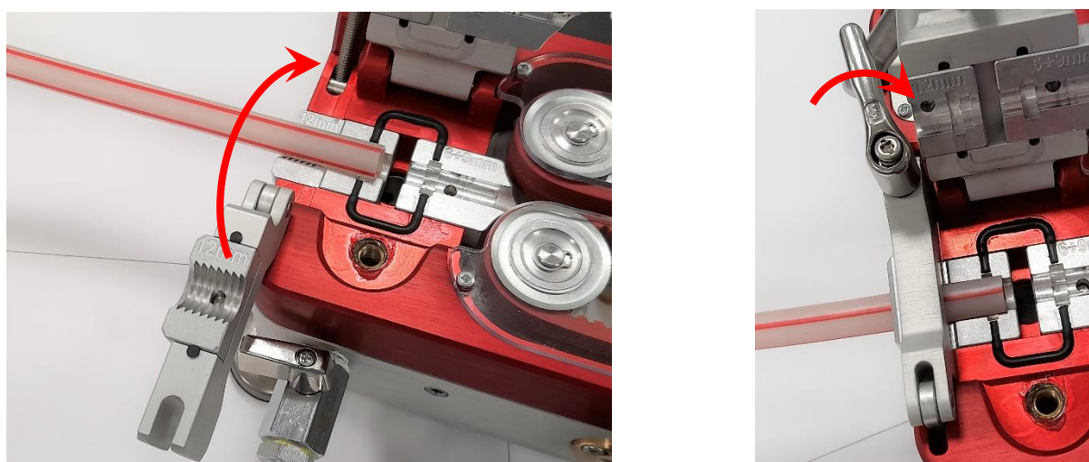
Figure 6: closing the minitube fixing clamp
