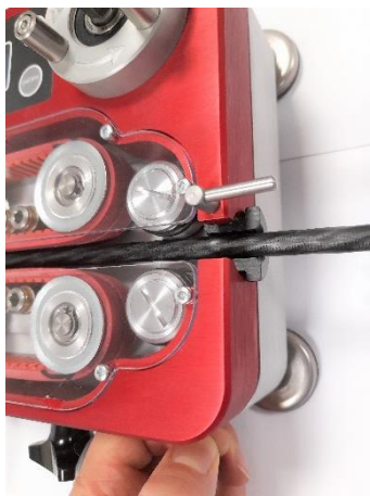
Figure 25: pulling the meter counter wheel opening lever to insert the cable
