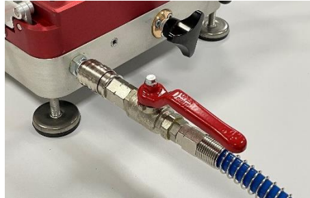
Figure 11: connecting the air hose to the compressed air connector
