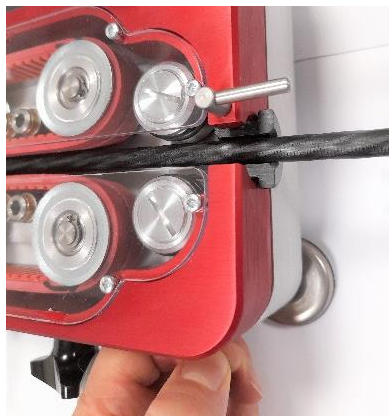
Figure 21: pulling the meter counter wheel opening lever to insert the cable
