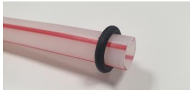
Figure 5: duct gasket insertion.
