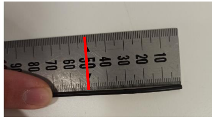
Figure 31: cutting the linear gasket.
