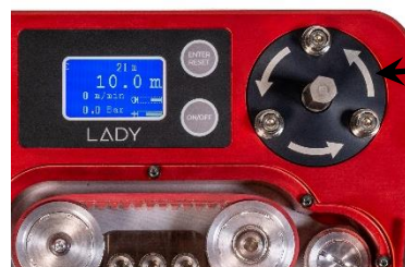
Figure 13: Direction of rotation of the electric screwdriver spindle
