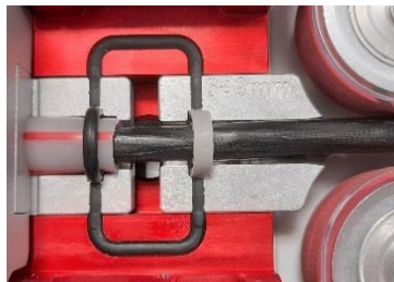
Figure 20: positioning the gaskets with cut facing down
