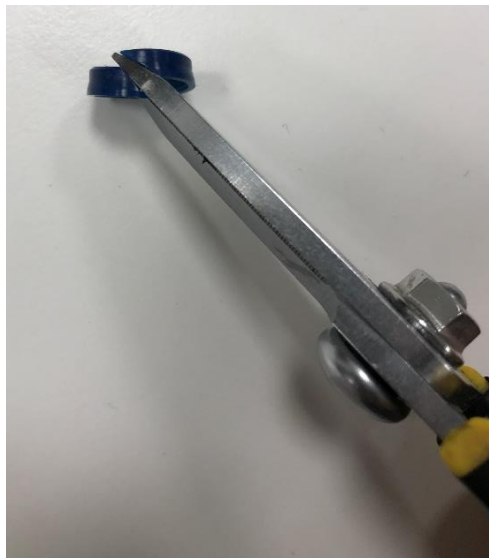
Figure 18: cut gaskets diagonally.
