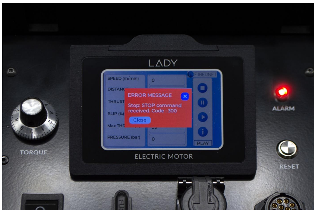
Figure 9: STOP Command Received error.
