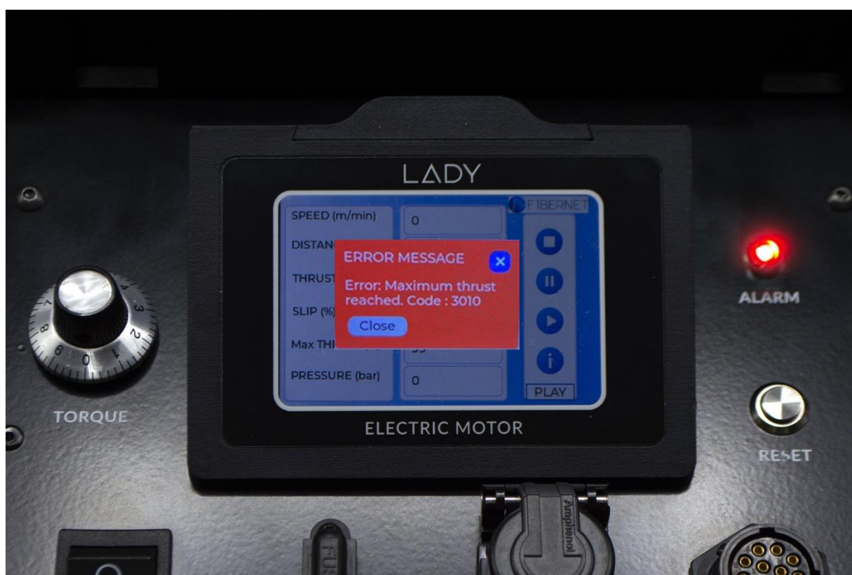
Figure 8: Maximum Thrust Reached error.
